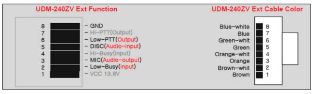
Cable UDM-MaxCable UDM-240ZV Interface cable hand-made to work with Maxon TM & MDM Series Mobiles \$ 25 \$ 40
