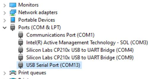
3. Run the ACC-916EX programming software. Before selecting the port number, plug the cable into the radio. Check the LED illumination on the radio while plugging the cable in. If it **does not blink** the radio has gone into programming mode. While in this state, simply select the port number from the menu and read/write to the radio. Ignore any pop-up windows stating to reset the power.
