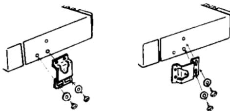
**E.** Connect the DC power supply cord to the radio. If necessary, the power supply cord may be connected before mounting the radio unit to the radio bracket.
