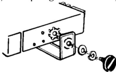
**NOTE** - Depending on the location where the radio unit will be mounted, it may be more convenient to install the microphone bracket before installing the radio unit into the radio bracket.
