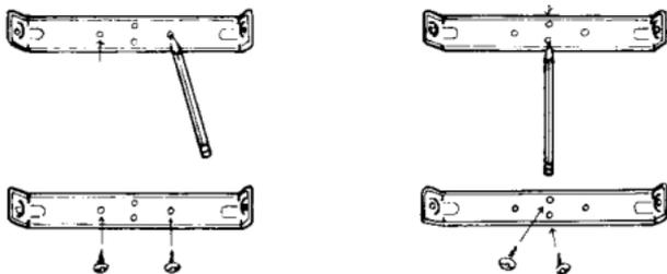
**NOTE -** Before drilling holes in the vehicle, verify that there is nothing that could be damaged or get in the way by drilling and putting screws in this location. It is better to use existing passages in the dashboard, trunk, and floor for the routing cable, thus avoiding excessive drilling.
