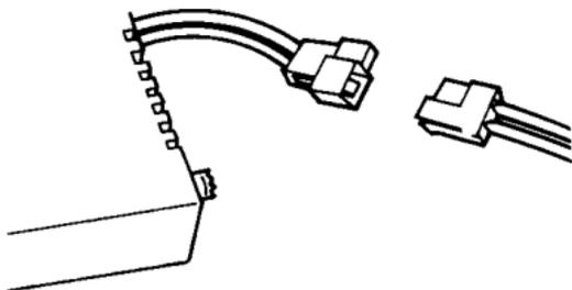
F. Push the modular microphone connector into the microphone jack (located in the front of the radio unit) until a click is heard.
