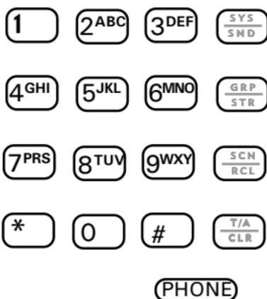
**Phone + SND "Send"** - Transmits the telephone number entered or recalled from memory on the radio's LCD.
