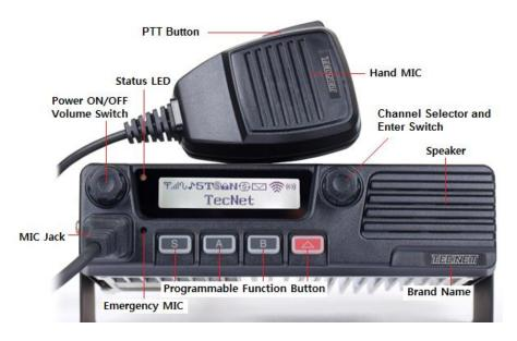
To prepare the Slave radio for receiving the new program, press and hold PTT on the hand microphone then turn the radio on using the Power ON/OFF Switch. When the display shows "LINE CLONE TX", release the PTT button. Rotate the channel selector to change it to "LINE CLONE RX". Next momentarily press the Channel Selector in to set.
