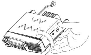
2. Next, turn the radio upside-down and insert a flat-head screwdriver into the holes of the chassis and tilt it in the direction as shown by the arrow. Do this on both holes to release the panel.
