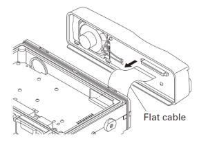
4. Plug the flat cable into the new front panel and clip the panel onto the chassis by installing the top of the panel first. Snap the bottom on making sure it is fully inserted onto the chassis.
