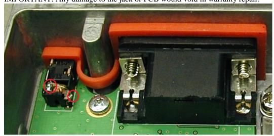
Note: External audio may also be obtained through the 15 pin connector on the radio.
