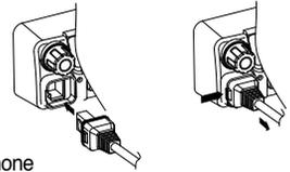
Figure 1-2) Installation and Removing of the Microphone
