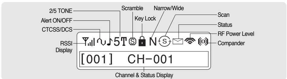
Figure 5-2) TM-2000 / TM-8000 Series LCD Indicator
