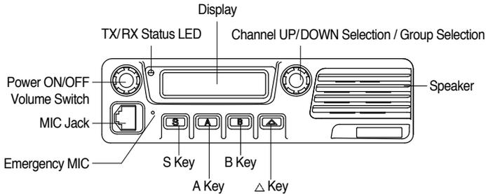
Figure 5-1) TM-2102 / TM-2402 / TM-8102 / TM-8402 Front Panel
