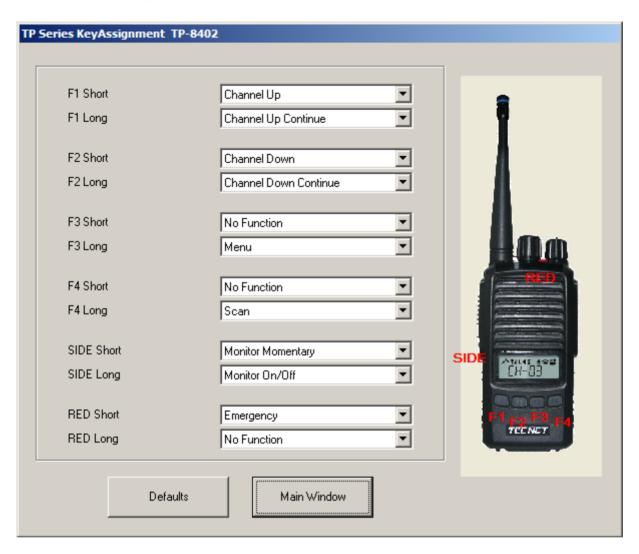
This window designates the function of each button on the radio. Please note that each button can perform a maximum of two different functions based on a short or long term press of that button.
