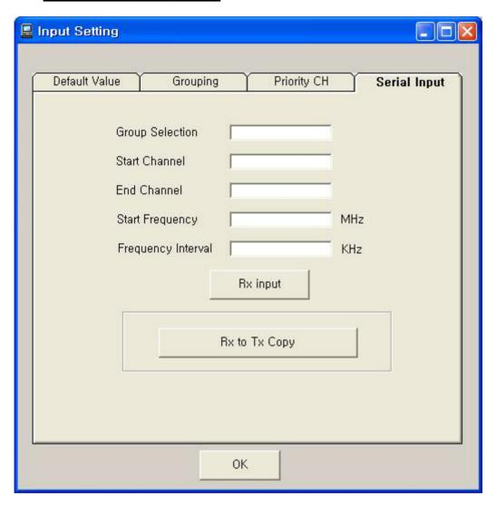
This window is for inputting frequency continually by same frequency interval.
