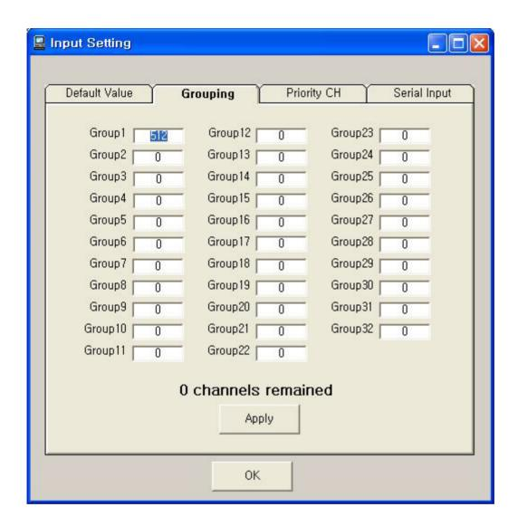
This window is used to assign channels to a group. Total number of channels (aggregate of groups) cannot exceed 512 channels.
