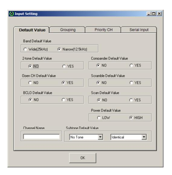
When inputting TX and RX frequency, the default setup values are inputted automatically for Band, 2-tone, Open CH, BCLO, Compander, Scramble, Scan, Power, Channel Name, and Subtone (sub-audible). When there are values already inputted, they are not affected.
