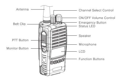
Note: Radio with orange keypad denotes TP-8000R series w/ Recording Capabilities
