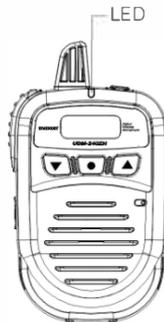
**\*Note: For vehicle charging, 12V Adaptor output should be 5V 800mA.**
