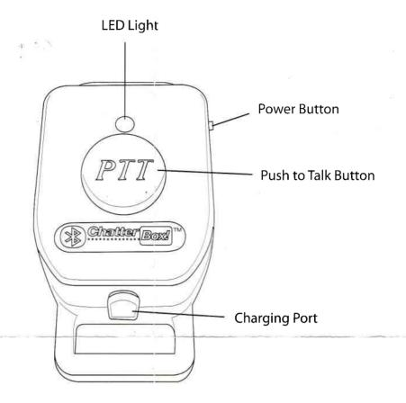
Powering ON wireless PTT button: Press and hold POWER button for 2-3 seconds until Blue LED light illuminates
